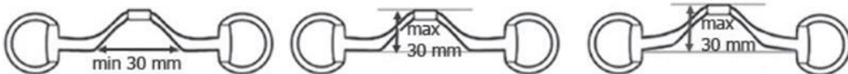
Figure 121.2: Measurement of tongue relief for a snaffle bit. The widest part of the deviation must be where the mouthpiece contacts the tongue and must have a minimum width of 30 mm (left). The maximum height of the deviation is 30mm from the lowest part of tongue side to the highest part of the deviation (center and right).
